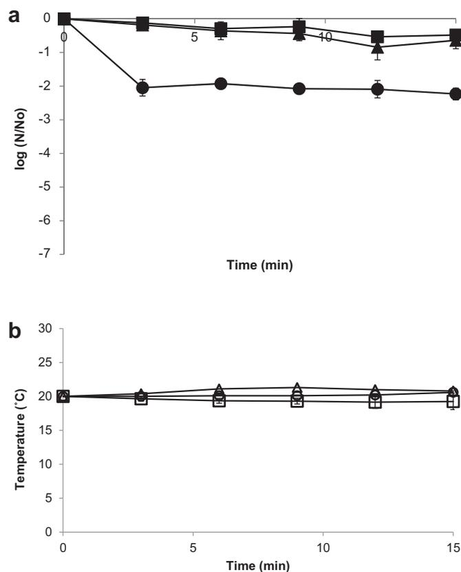
**Fig. 4.** a) Inactivation of *E. coli* in (▲) carrots, (■) lettuce and (●) tomatoes using ozone at 5 ppm; (b) profile of temperature during disinfection of vegetables with ozone, (▲) carrots, (□) lettuce and (○) tomatoes. Each experiment was run at least in duplicate and at least five samples were analyzed in each experiment. Initial count was  $10^7$ – $10^8$  cfu/ml.
