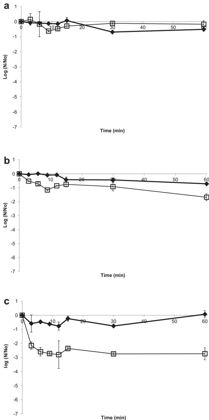
**Fig. 3.** Inactivation of *E. coli* in a) carrots; b) lettuce; and c) tomatoes using ultraviolet light at two working distances: (◆) 70 cm: total fluence 0.65 mW/cm<sup>2</sup> and (□) 31 cm: total fluence 1.6 mW/cm<sup>2</sup>. Each experiment was run at least in duplicate and at least five samples were analyzed in each experiment. Initial count was 10<sup>7</sup>–10<sup>8</sup> cfu/ml.
