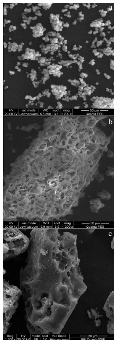
Fig. 1. SEM microstructure of three samples: (a) NRS, (b) GRS, and (c) RRS.
