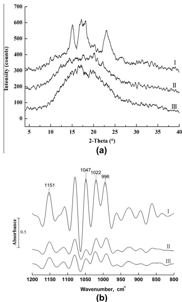
**Fig. 3.** (a) X-ray diffraction patterns of three samples: NRS (I), GRS (II), RRS (III); (b) FTIR deconvoluted spectra of three samples: (I) NRS (II) GRS (III) RRS.
